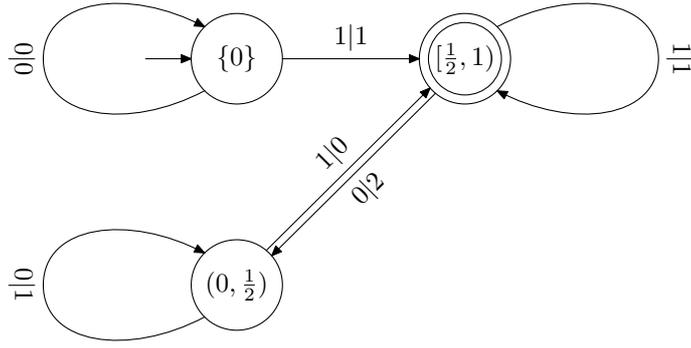
FIGURE 3. Right-To-Left-Transducer for  $\alpha = 3/2$ .
