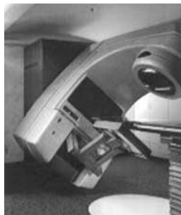
Figure 1. A linear accelerator used for external beam radiotherapy treatment.
